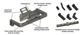
Figure 2: Base frame, rotatable spacers, and linear rail to attach modules.
