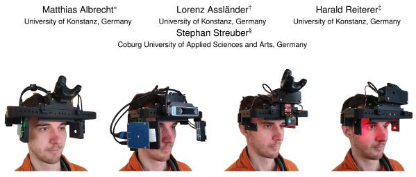
(a) Parallel LCDs and HTC Vive tracker (b) Angled LCDs and Intel RealSense (c) LED sticks, transparent OLED dis- (d) LED matrices without extra tracking play and HTC Vive tracker module
