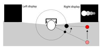
Figure 6: Top-down view of peripheral out-of-view visualization. A movement of an object in the rear back of the user (depicted as red circles) leads to a change of position and scale of the rendered sphere around the user's head (depicted as black circles), which can be seen on the right display. The gray area depicts the rendered field of view of the cameras, not of the user.
