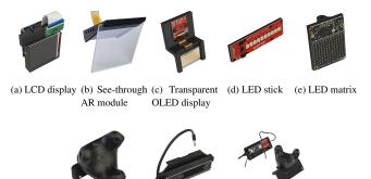
(f) HTC Vive (g) Intel T265 (h) Arduino tracker tracking camera with IMU and optional tracker
